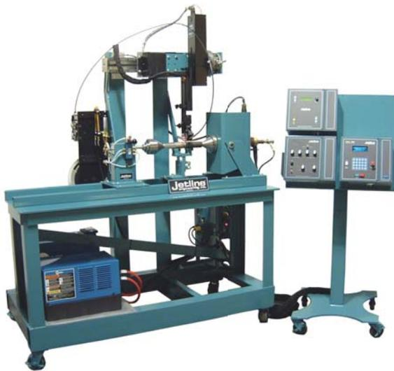
Benchmaster GTAW System 9500 System Control, ALC-401-6 arc length control, and MO-150-5S mechanical oscillator. Controls are mounted on a moveable podium for easy access.
