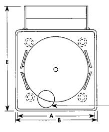
Apparatus Well Includes: Torch Water in and out, Torch Gas in, Chamber Purge, 115 v in.
