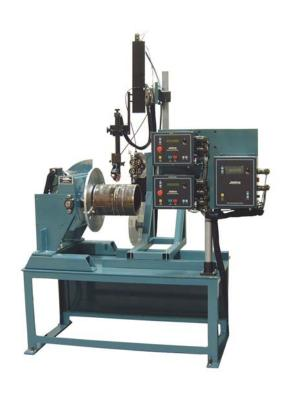
Benchmaster GTAW System with JP-500 positioner, 9640 rotation control, ALC-401-6 arc length control, and CWF-20 precision cold wire feed.
