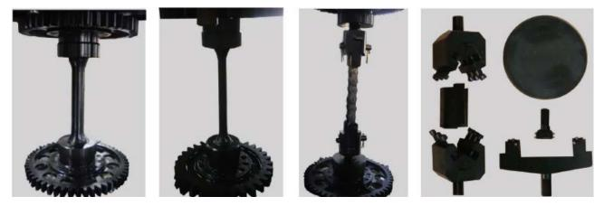
Tensile grips for round specimen & flat specimen / Compression platen / 3 points flexure fixture
