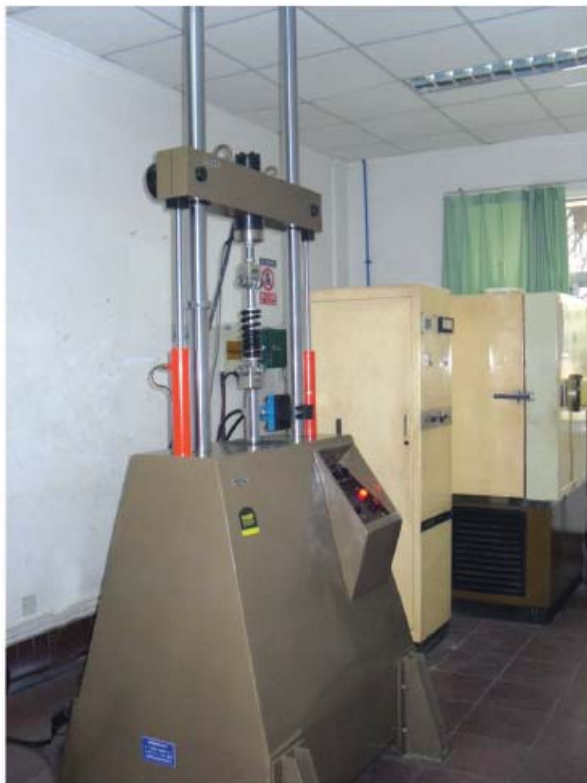
100KN load frame for absorber test
