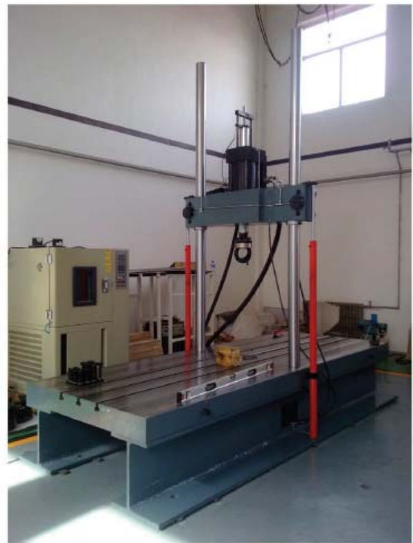
100KN for dynamic bending test with 'bed'
