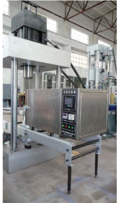
500KN load frame for low temp. test
