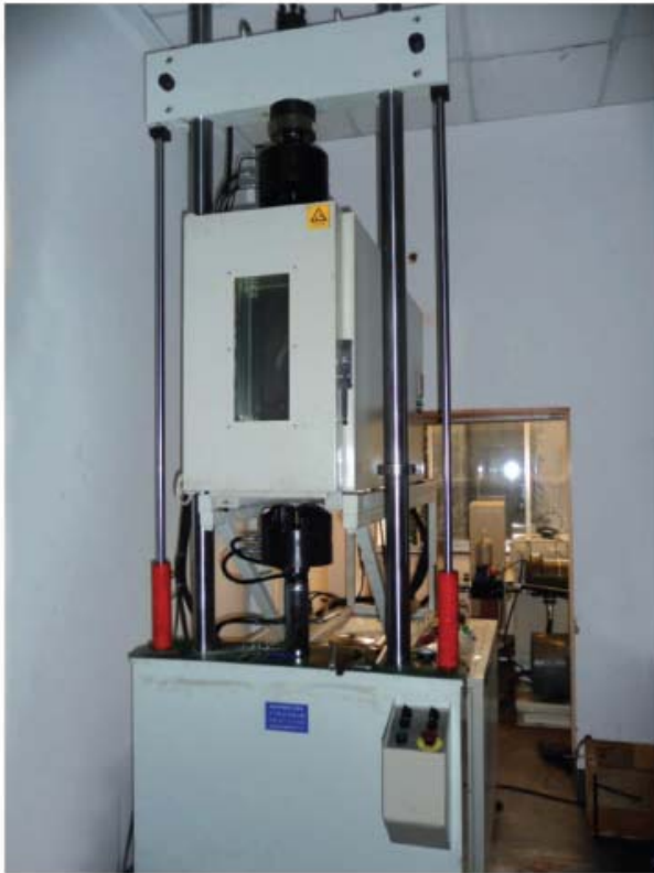
100KN load frame for high temp. test
