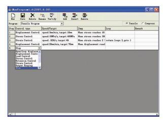
MaxProgram Editor possess of multi-kinds full digital control modes, i.e Displacement control, Stress(Load) control, Strain (Deformation) control, Low cycle control. Users can edit the most complex and logical procedure by MaxProgram Editor. The combination of above functions can meet all kinds of routine test purpose.
