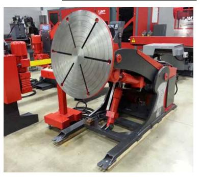
Hydraulic Elevating Welding Positioners
