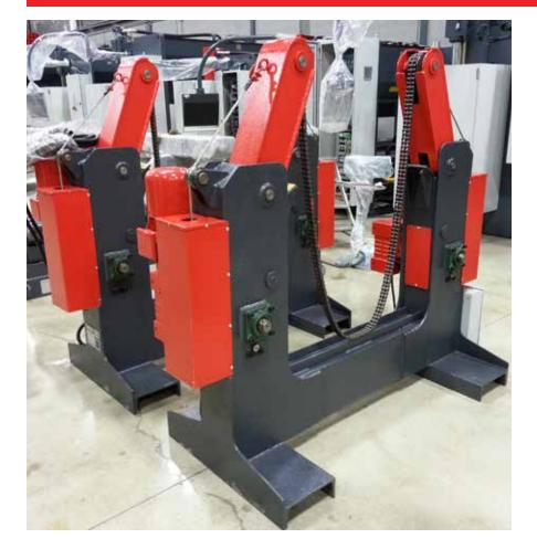
Chain driven beam rotators can rotate a beam or other long work piece to position it for welding.
