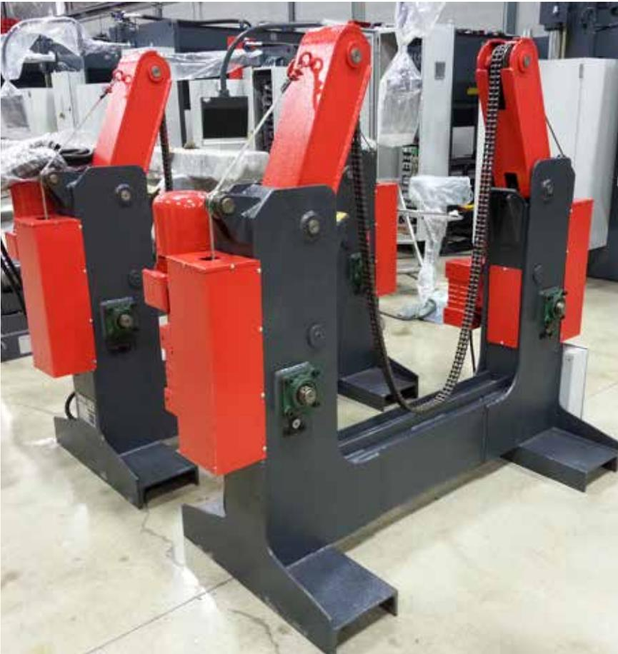
Chain driven beam rotators can rotate a beam or other long work piece to position it for welding.
