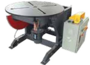
Turntable welding positioners allow work pieces to be revolved 360° and pivoted 90°, keeping the welding torch in one position as the work piece moves. This eliminates operator fatigue, increases productivity and generally produces higher quality welds.
