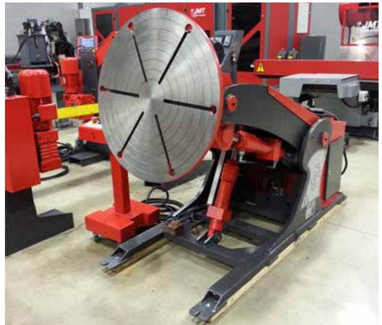
Hydraulic Elevating Welding Positioners
