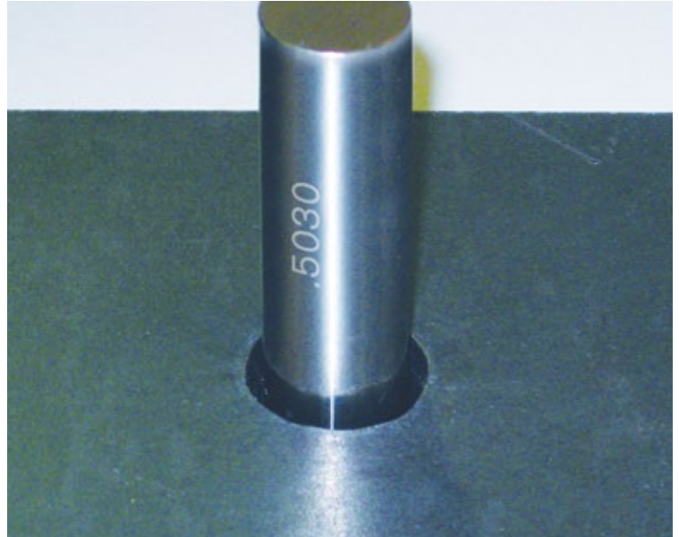
1/2" hole without True Hole technology cut with HPRXD® Plasma
