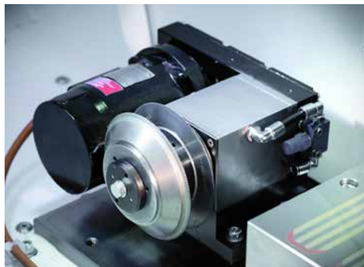
PA-TL28 for surface grinding and grinding of standard profiles with small radii and high accuracies. Overhung-mounted, fixed dressing wheel with adjustable angular position.
