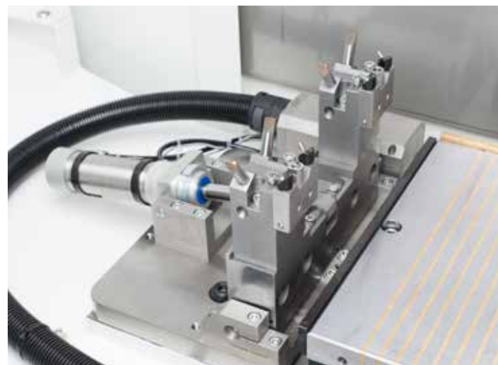
Folding dresser for peripheral, lateral and profile dressing. Grinding wheel and protective hood cannot collide with the dresser. A roughing and a finishing station.
