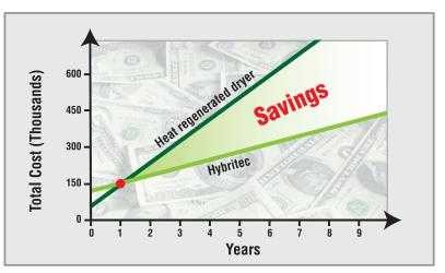
Graph shows a 3000 scfm system running the desiccant dryer for 7 months of the year, 8760 operating hours per year at \$0.10/kWh
