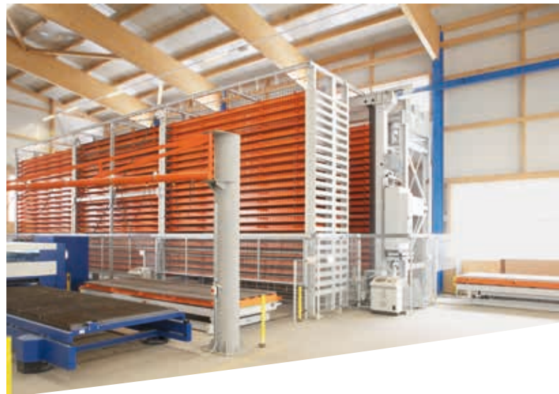
UNILINE: In-line storage systems for effective material supply to processing machines and for commissioning.
