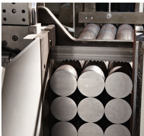
Hydraulic bundle clamping device at the outfeed side.
