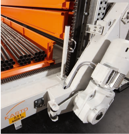
Lifting beam with cassette for long material and lifting gear drive.
