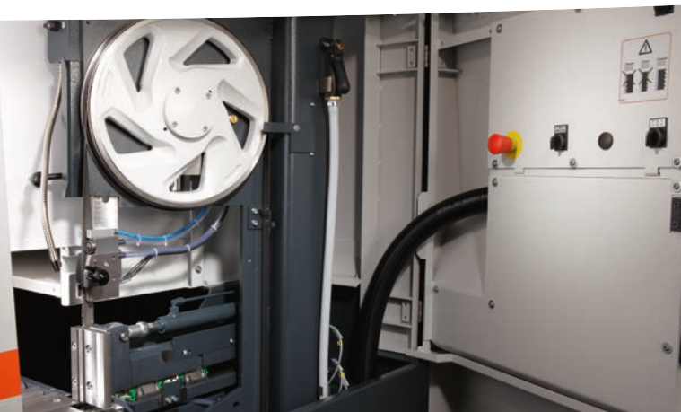
Easy exchange of saw blade.
