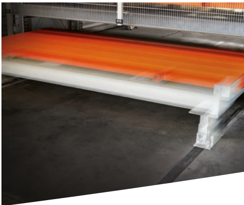
Manually movable lateral carriage for loading at the rear side of the system (accessory).
