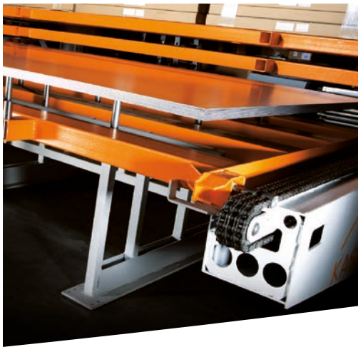
Storage support for free-lift of the loading goods (accessory).
