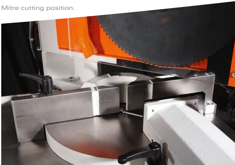
Clamping vice with counter clamping vice.
