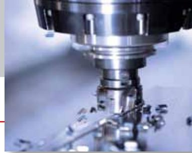
A high power spindle for extreme roughing operations on a highly rigid ram enabling the maximum use of the output with the maximum extension.
