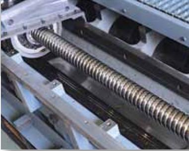
A massive cast iron cross beam on a highly precisely designed support. The drive of the nut for the ball screw is integrated in this support.
