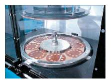
• Each Drive System is mounted in fully sealed taper roller bearings to allow the smooth running of the lap plates.
