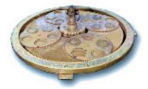
The 3 way drive concept has the top and bottom plates and sun gear running with independent drives with Variable speeds and fully reversible operation.
