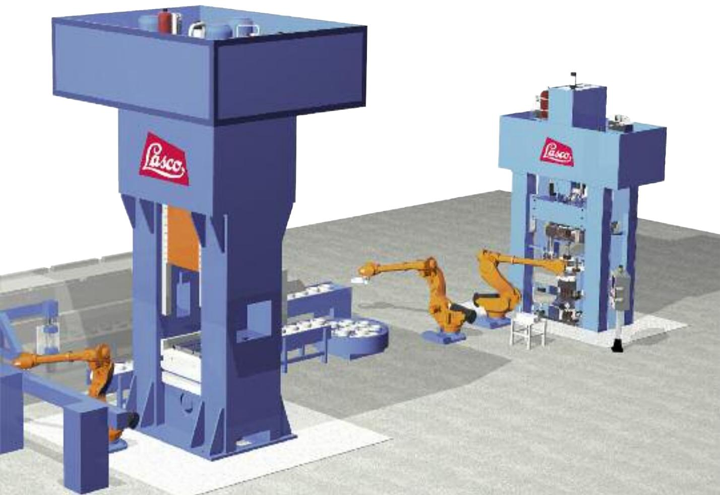
Schematic of two inter-linked LASCO units VPE 500 and MPP 400 with automation devices.
