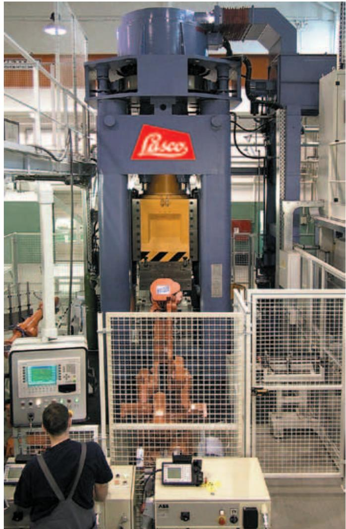
*LASCO screw presses with frequency converter drive are in use worldwide. In the illustration, racks for automotive steering racks are being produced on an automated SPR 1000.*
