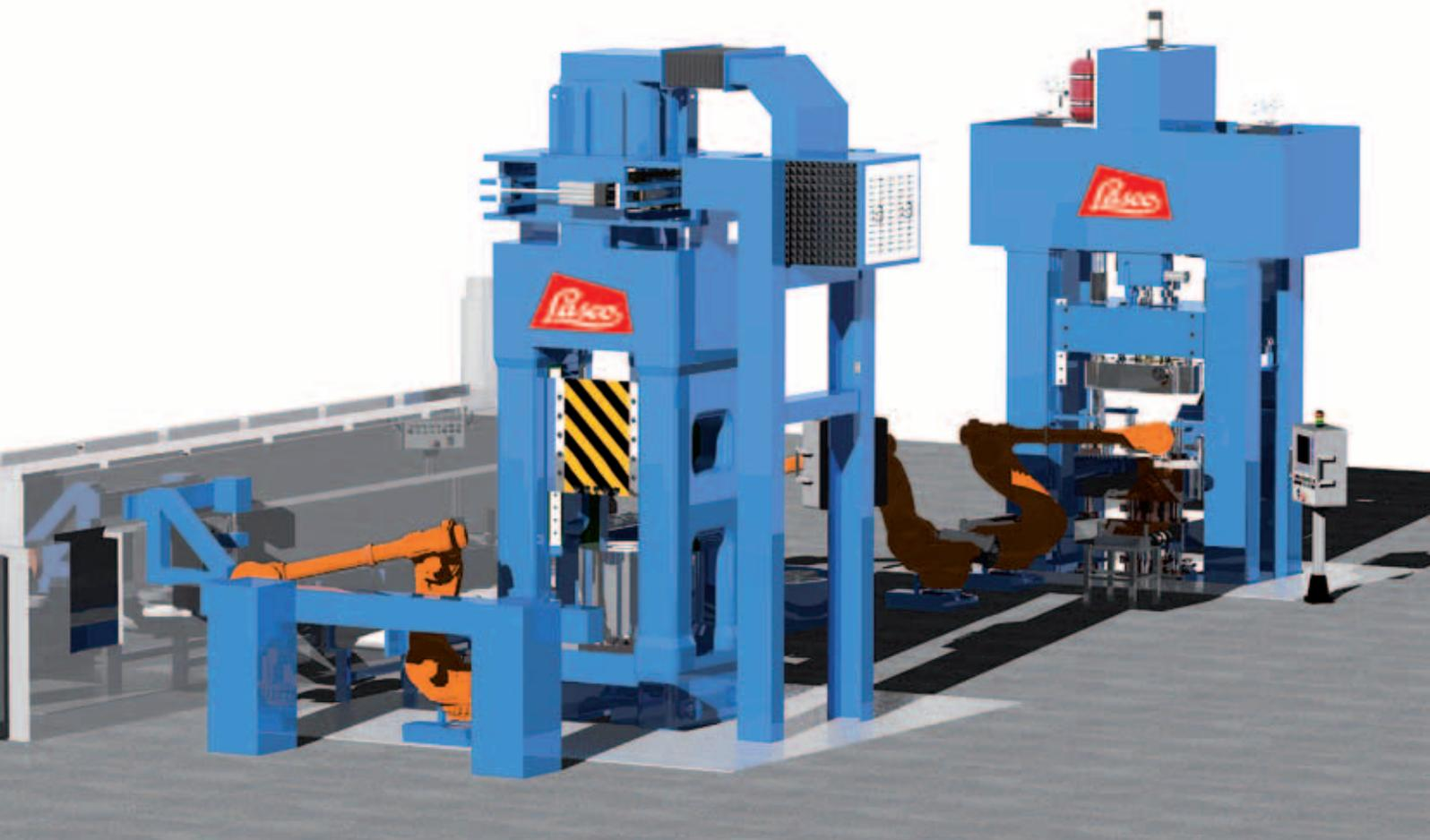
*Schematic of two interlinked LASCO units SPR 630 and MPP 400 with automation devices.*
