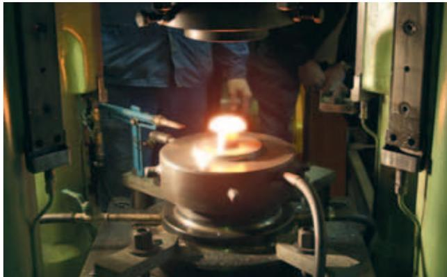
Production of connecting elements on an SPR 315.
