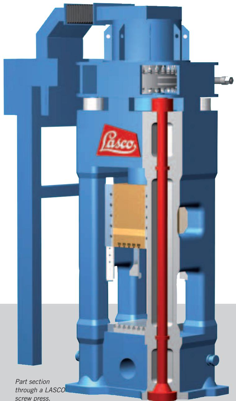
*Part section through a LASCO screw press. The compound frame, pre-stressed with tie rods, is optimized for complex forming requirements.*
