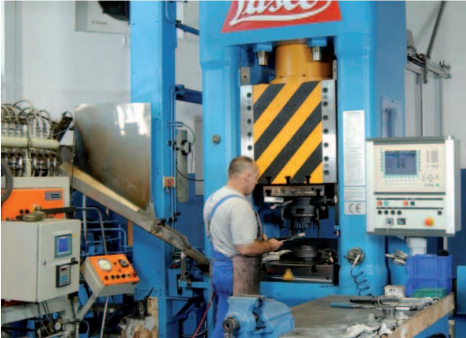
An SPR 400 screw press used for production of electric armatures for railroad vehicles. The preheated blanks in the furnace (left) are fed to the machine through a chute.
