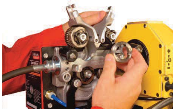
Fast, tool-less changeover of drive rolls.
