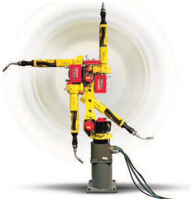
The AutoDrive® series maximizes robot arm speed and work envelope.
