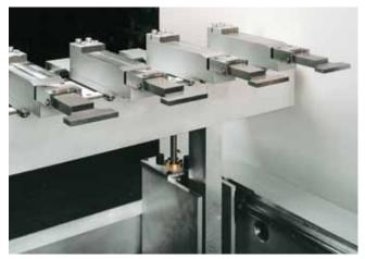
*Two-axis backgauge (X-R) with manual Z-axis. Pneumatic clamping for finger positioning on PPEB-5*
