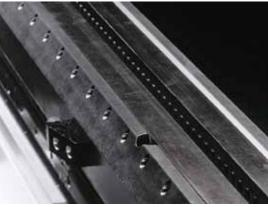
Hydraulic clamping system on table PP3160
