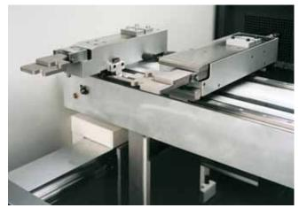
Five-axis backgauge X-R-Z1-Z2-X' on PPEB-8 and PPEB-EFL
