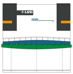
**CADMAN® Control/Software**: The LVD CADMAN® Touch press brake control assures first time bend angle results by the automatic application of the exclusive CADMAN angle correction database. Previous bending data experience on specific tools and materials are cross-referenced and automatically applied.
