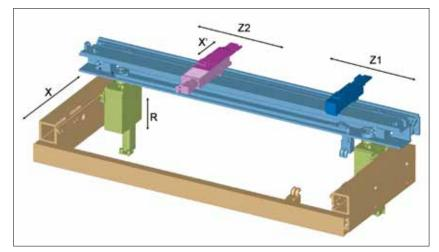
Whether you require a basic twoaxis backgauge or a more complex system to allow multi-bend set-ups and the production of taper bends, LVD can offer a solution that takes the guess work out of all axis position calculations by using the CADMAN advanced software.
