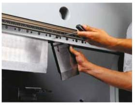
Self-seating manual clamping system PP3090
