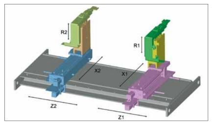
Six-axis backgauge X1R1Z1-X2R2Z2
