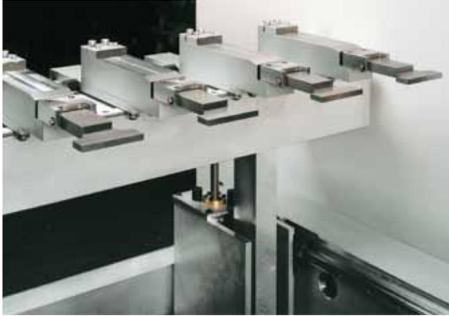
Two-axis backgauge (X-R) with manual Z-axis.
