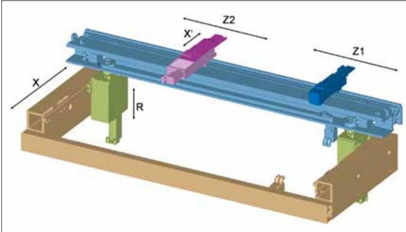
Five-axis backgauge X-R-Z1-Z2-X' (standard on PPEB-8 and PPEB-EFL)
