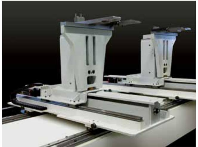
Six-axis modular backgauge X1R1Z1-X2R2Z2 for 500T & 640T
