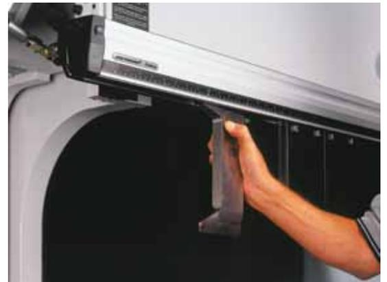
*Self-seating hydraulic clamping system PP3100*
