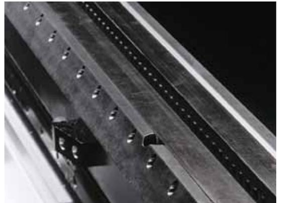
*Hydraulic clamping system on table PP3160*
