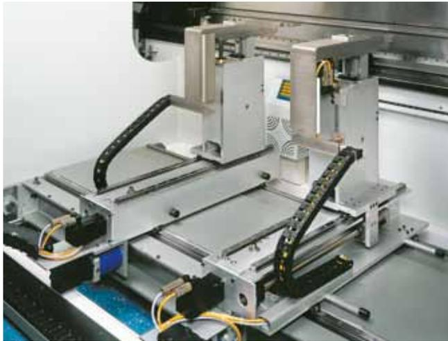
Six-axis modular backgauge X1R1Z1-X2R2Z2 up to 400T
