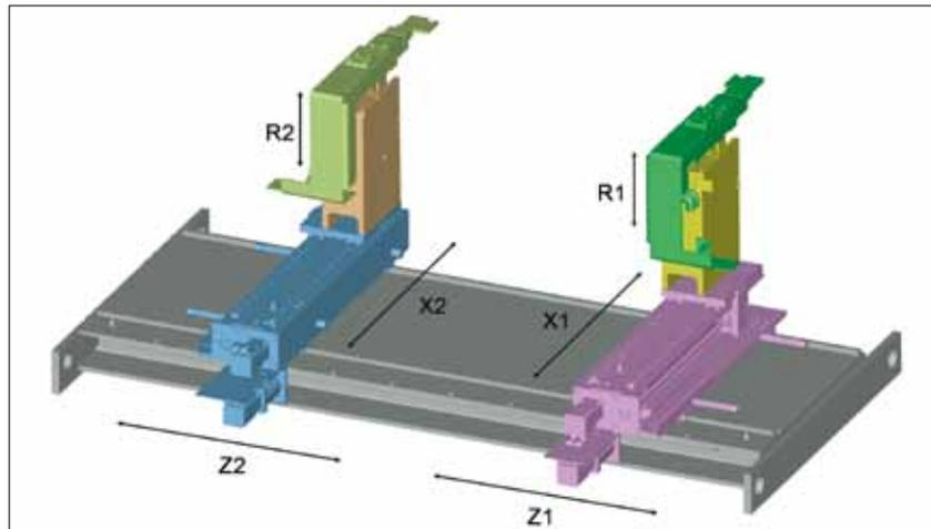
Six-axis backgauge X1R1Z1-X2R2Z2
