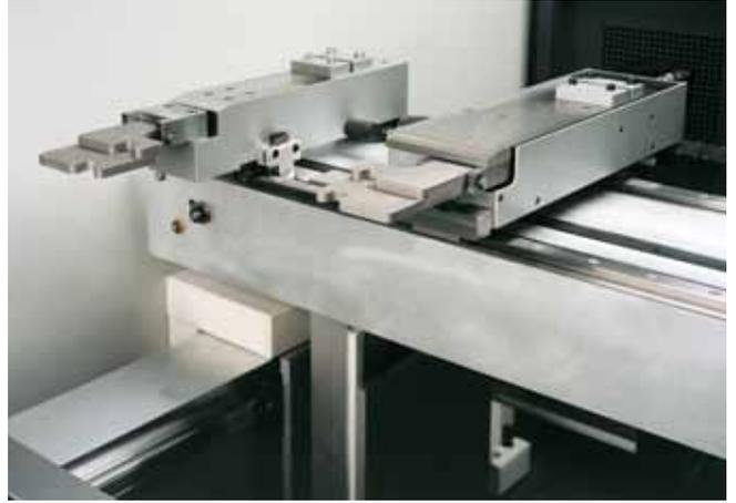
Five-axis backgauge X-R-Z1-Z2-X' on PPEB-8 and PPEB-EFL
