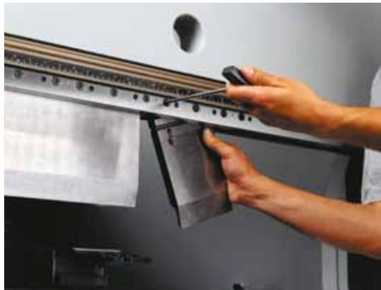
*Self-seating manual clamping system PP3090*
