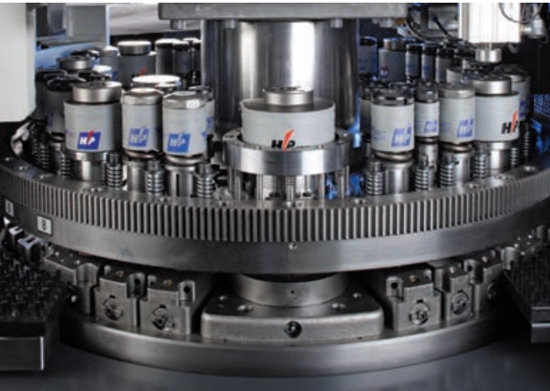
A large capacity turret features 48 stations.
