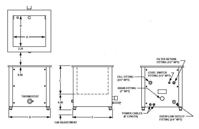
NOTE: Model CT09-P1K is illustrated in this drawing, optional work station base not shown.
