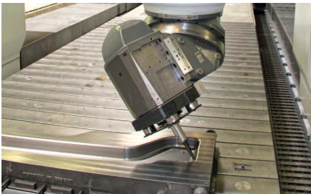
Universal milling head with taper HSK 100
