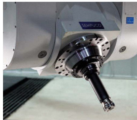
2-axis swivel head with 9,000 rpm
