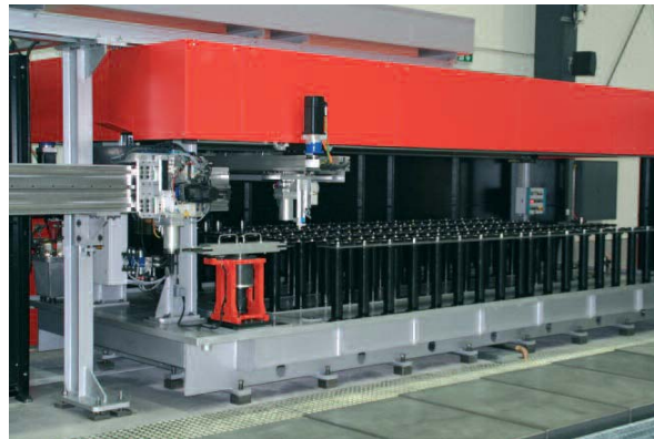
Tool magazine HSK-A 100 with 200 tools
