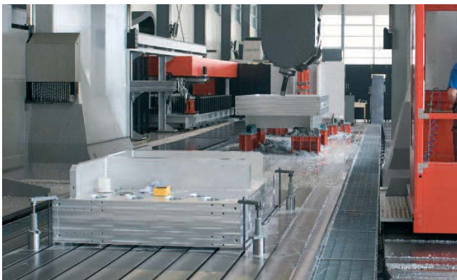
The flush embedded machine table is perfect for heavy parts
