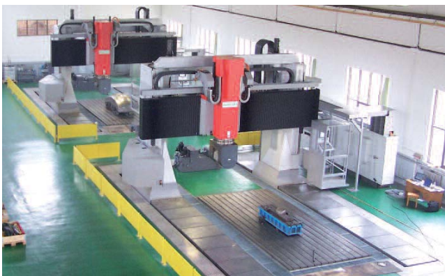
Floor-running gantry machine in row
