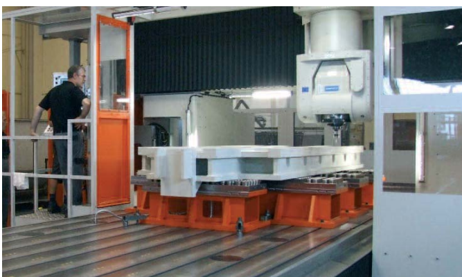
matec-40 P with 2-axis swivel head
