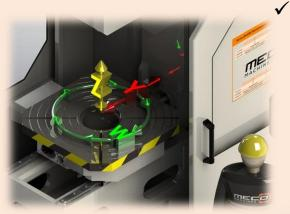
**3 AUTOMATIC AXES.** Thanks to the electronic control systems of last generation that have been incorporated in this model for its three axes is achieved greater precision and a higher degree of automation. The machine can work in automatic mode, so that the operator can simply handle replace the part once the machine has finished the process of pre-programmed machining. Undoubtedly, the MECO broaching machines are designed to increase the production capacity of our customers.
