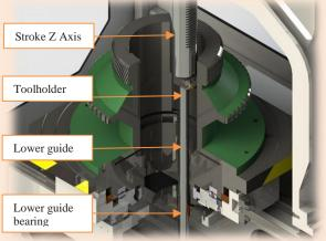
**BLIND SAMPLES.** Disassembly the guide bar and programing properly the limit switches, the tool can enter in blind parts and machining grooves or keyways.
