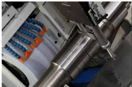
**Morara's MH 3000** (formerly GCH E/E 3000 CNC **rail road axle grinder**, with the work piece load of 2500 Kg and the double wheels (right and left) with 20° angle approach, complete the machining in a single set-up.
