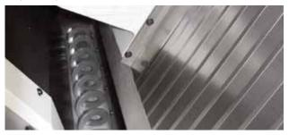
Coolant tank with chip flushing system
