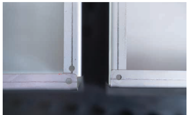
Example and details of a bent panel without corrections (left) and with corrections imported from the TMDB (right)
