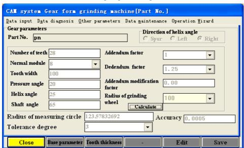
Profile computing module for grinding wheel - Profile and Lead modification. This module serves to gather data in order to generate the correct wheel profile through an editable series of dressing cycles using the on-board dressing wheel system. Based on data entered about the workpiece and special requirements on gears to be machined; including profile, lead modification and fillet curve parameters, the profile of the grinding wheel can
