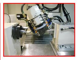
The working principle of this machine is form grinding. The profile of the grinding wheel is modified via on an on-board wheel dressing system utilizing a diamond
