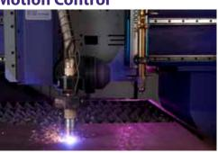
Powerful dual-side SERVO motors combined with low backlash planetary gear boxes and helical rack and pinion drives move the gantry of the HORNET XD along the X and Y axes at speeds up to 1,000 IPM (25.4m/min).
