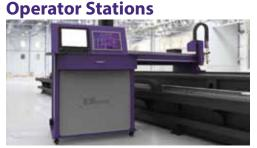
The HORNET XD comes standard with a rotatable attached operator station. The HORNET XD is also available with a remote pedestal operator station. Each operator station includes a 15" LCD touch-screen monitor, industrial keyboards, mouse, and E-Stop button. If needed, the operator station also includes an oxy-fuel operator control panel and a dust collector Start/Stop button.
