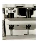
Vertical head adjustment is accomplished simply. A single adjustment of the outside drills makes it possible to use drills of different lengths. High-compression "hold-down" and stripper bar along with a fixed 4-1/4" (108mm) drill spacing provides perfect accuracy and eliminates spacing errors.
