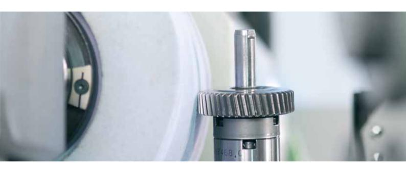
G 160 generating gear grinding machine
