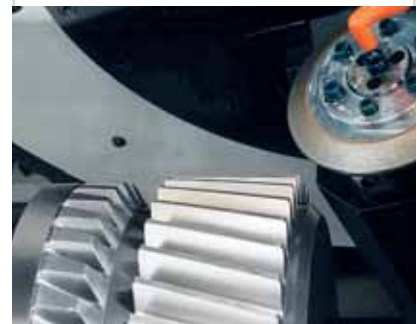
Grinding large module gears with electroplated CBN grinding wheel
