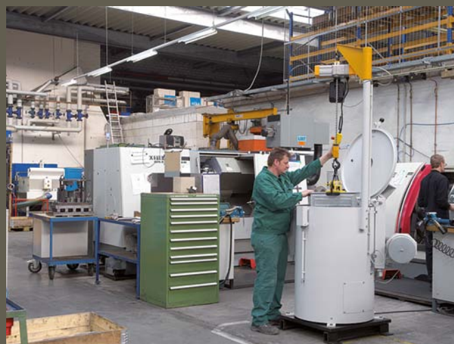
▲ POLAR C centrifuge for de-oiling of parts in boxes; with swing-jib
