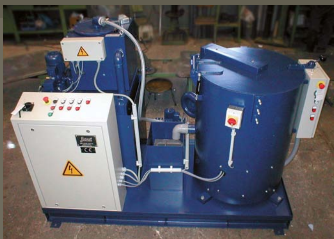
▲ POLAR C for de-oiling of parts and swarf; with oil cleaning centrifuge and oil tank
