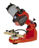
Features include: an offset 10 degree tilting vise for correct corner (or leading edge) angles on chisel cutters, a cutting length adjuster, easy-to-read vise and head angle scales and a chain-centering feature that ensures both left and right cutters are ground to equal lengths and angles. With the added feature of a hydraulic chain clamp vise, this automatically locks the chain when the grinding head is lowered and can reduce sharpening time by as much as 50%!
