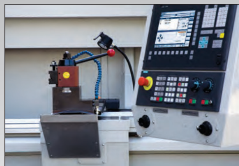
QC USA made Toolpost and Siemens 840Dsl control station
