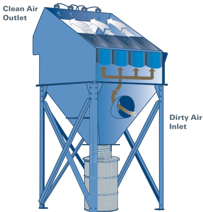
NORMAL OPERATION FOR CPC-3 THROUGH CPC-48 MODELS
