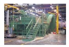
includes screen for media classification, conveyors and media storage hopper. Specially designed sound enclosure allows system to operate at 80 dba. OHD 9696 380 cubic foot capacity.
