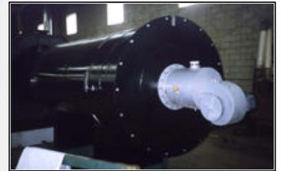
Optional Refractory Lined Combustion Chamber
