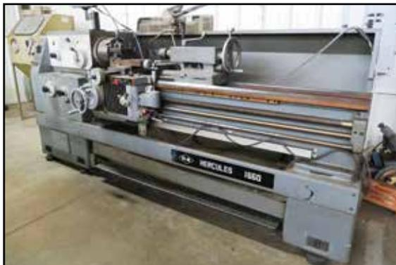
HERCULES 1660 16" X 60" ENGINE LATHE
