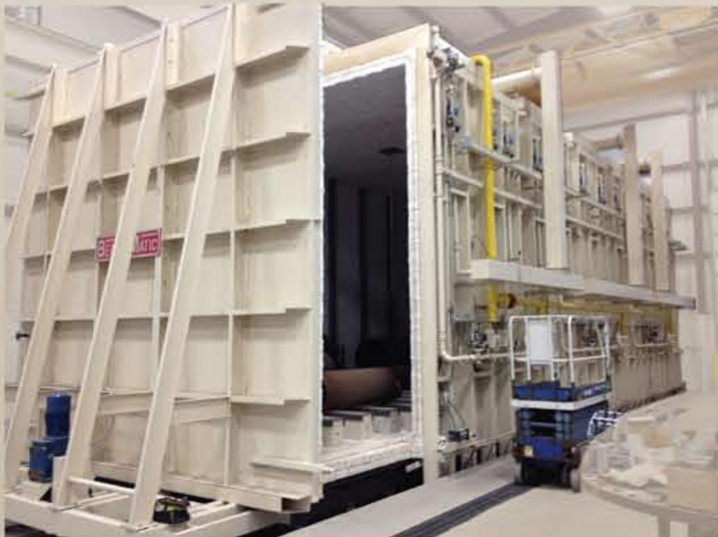
Carbottom Furnace capable of processing a 14 foot wide by 14 foot high by 45 foot long workload that weighs up to 80,000 lbs.
