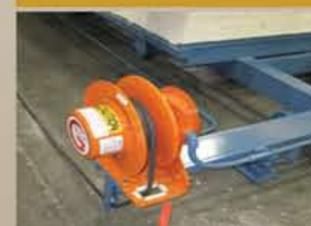
Car drive system with cable reel is required to drive the car in and out of the furnace for loading and unloading.
