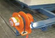
Car drive system with cable reel is required to drive the car in and out of the furnace for loading and unloading.
