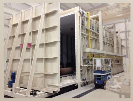
Carbottom Furnace capable of processing a 14 foot wide by 14 foot high by 45 foot long workload that weighs up to 80,000 lbs.
