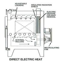
EXHAUST FLUE W/ ADJUSTABLE SHEILD AJUSTABLE AIR BAFFLES BELT DRIVEN HIGH TEMPERATURE RECIRCULATING FAN
