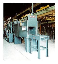
New 24"W x 36"D x 20"H multi-zone BeaverMatic unit combines temper furnace processing with a two chamber washer in one continous operation.
