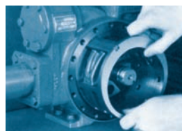
Easily replaceable liner restores efficiency.
