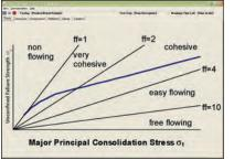
Flow Function for powder sample shows "non-flowing" to "very cohesive" behavior at low consolidation stresses and "cohesive" behavior at higher consolidation stresses.
