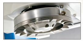
Close-up View of Vane Lid used for Flow Function Test.
