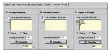
Data output from Flow Function test provides "Arching Dimension" and "Rathole" diameter. Data output from additional Wall Friction test provides "Hopper Half Angle".
