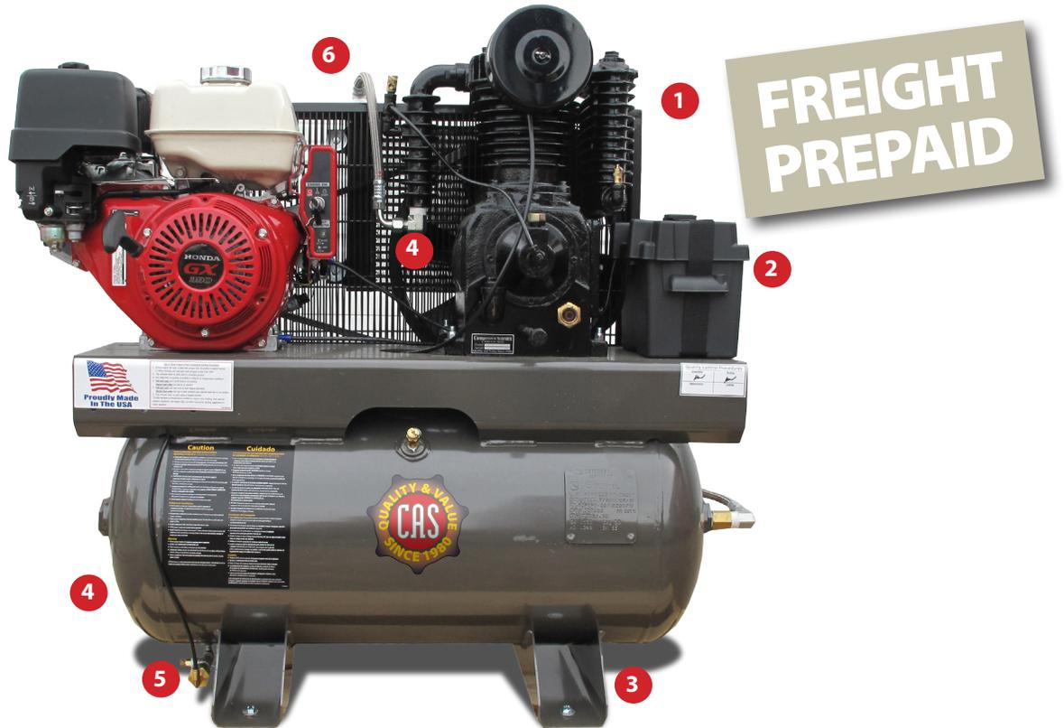
**1 Belt guard after cooler.** This cools the air before it goes into the receiver, so more moisture stays in the receiver rather than running to your air tools.
