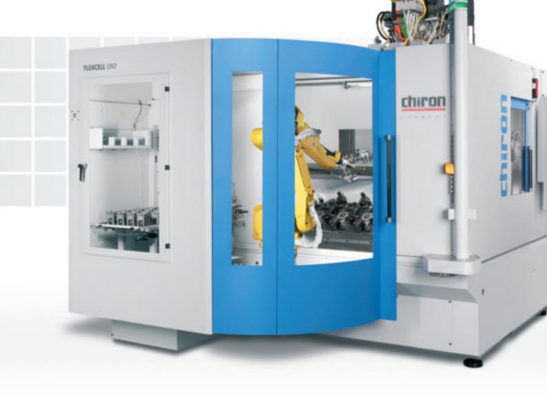
Machining center and robot cell as one unit – integrated automation in the smallest possible space: transported together, no separate setup, no need for additional alignment of the robot cell or for further protective devices.
