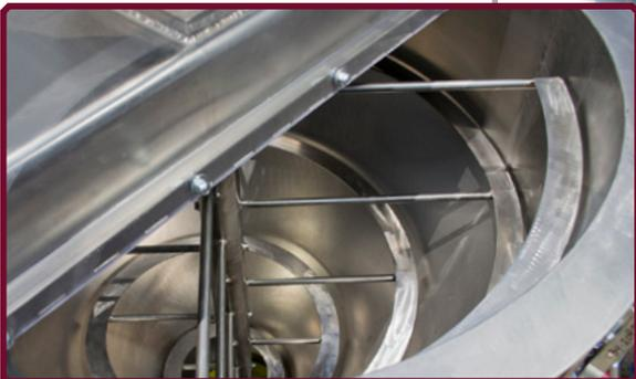
MIXING ACTION IS DEVELOPED BY A HELICAL SHAPED, SPIRAL MIXING RIBBON
