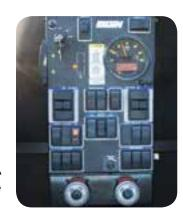
Elgin's Memory Sweep® system allows the operator to resume all previous sweep settings, even broom tilt (if so equipped), with one-touch control to enhance productivity and reduce fatigue. It incorporates a
