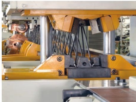
Medium-frequency welding group with four transformers each with 125 kVA and two inverters each with 300 kVA
