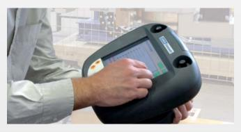
The ergonomics of the handheld operator panel is optimized for left or right hand operation.
